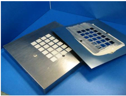
Lift off the metal mask.
